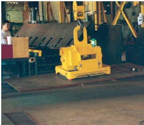
Auto-attach/release bail on this vacuum lifter allows for hands-free operation. Available as 6,000 pounds single pad or 12,000 pound dual pad units, these 33" square pads are designed for handling material in steel and aluminum mills.
