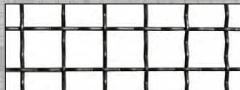
1-5/8" CENTER-TO-CENTER SQUARE 8 GAUGE WOVEN (1-1/2" SQUARE OPENING)
