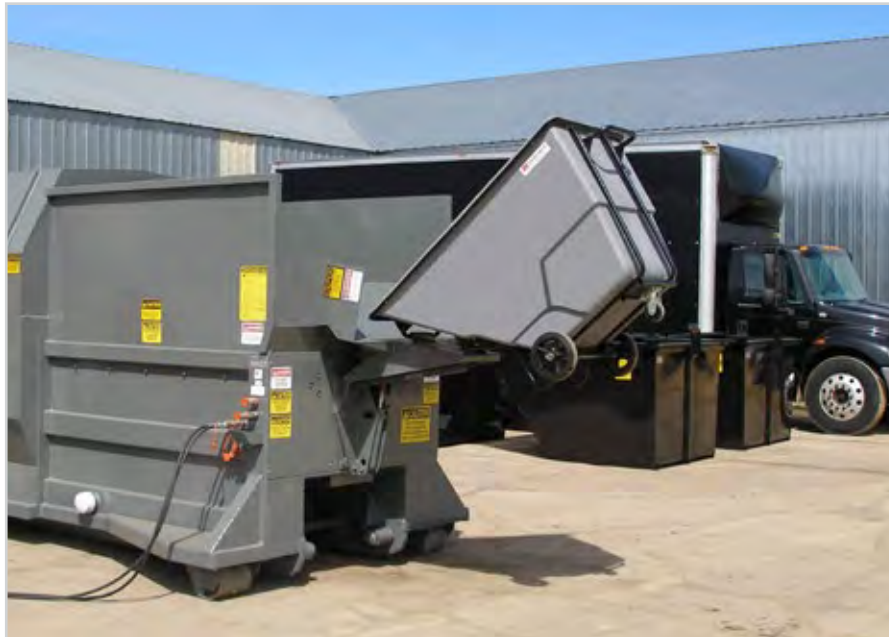
Akro-Tilts have 13-gauge metal lift handles which work with tilt cart dumpers.
